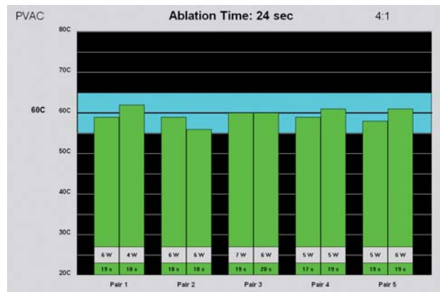
Figure 3: Example of generator display during ablation with PVAC, with temperature and power for each electrode, number of seconds each electrode is within 5°C of the target temperature during the ablation.
