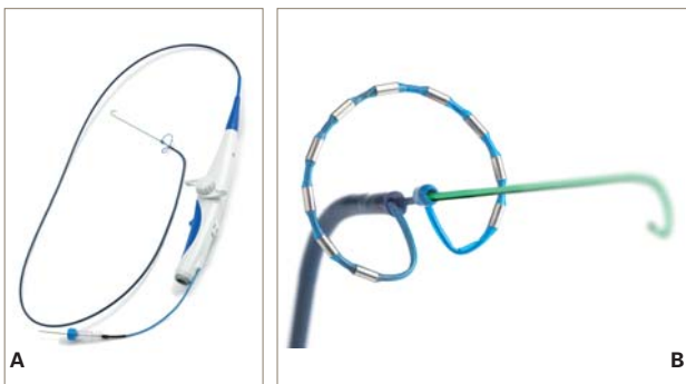
Figure 2: (A) PVAC showing 0.032" guidewire and control knobs on catheter handle. (B) distal portion of the PVAC showing ten 3 mm electrodes with 3 mm spacing.
